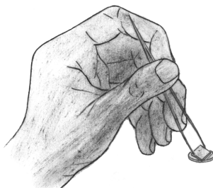
Figure 7.2k Securing Double-sided Tape to the Sample Disk
