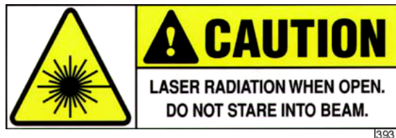
Figure 2.9c Noninterlocked Protective Housing Label
